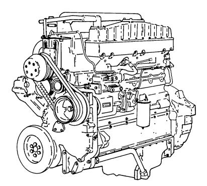
ENGINE, DIESEL, 6 CYLINDER INLINE, TURBOCHARGED, CUMMINS MODEL NTC-400 BC2 NSN 2815-01-156-6210
